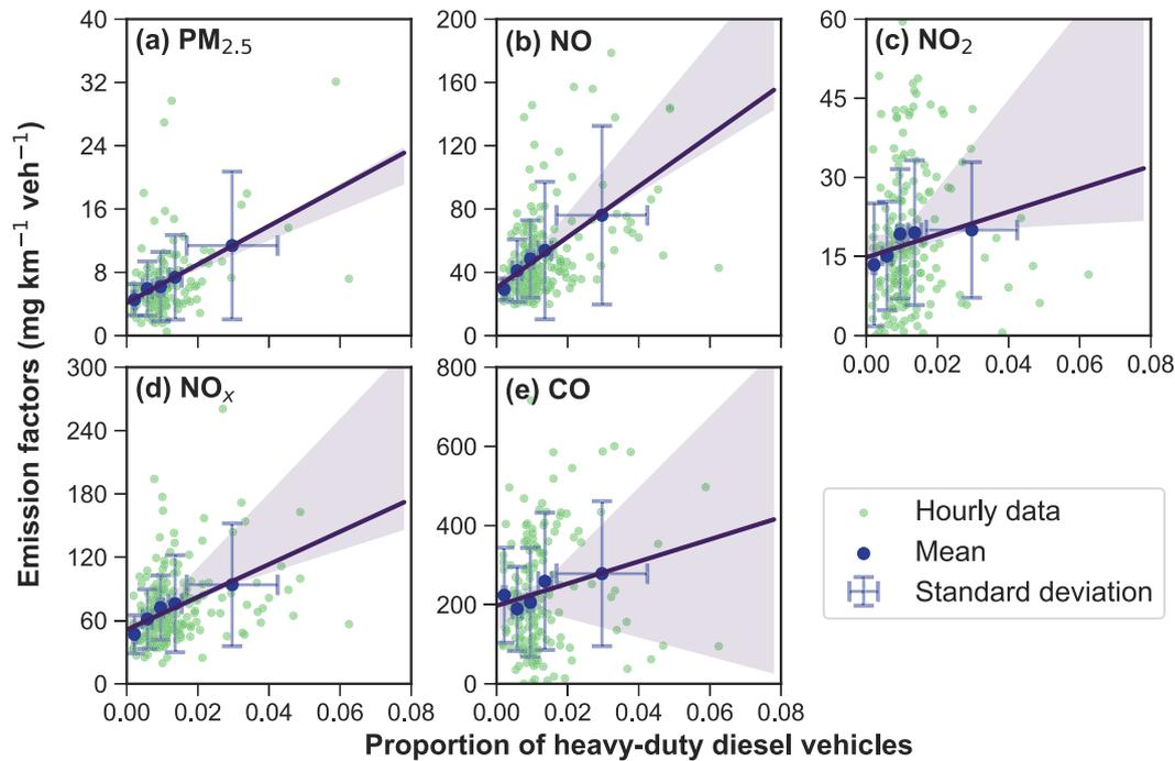
**Fig. 5.** Linear regressions between the average emission factors (a:  $PM_{2.5}$ , b: NO, c:  $NO_2$ , d:  $NO_x$ , and e: CO) and proportion of heavy-duty diesel vehicles (HDDVs). The fit lines were filled with 95% confidence intervals of regressions.
