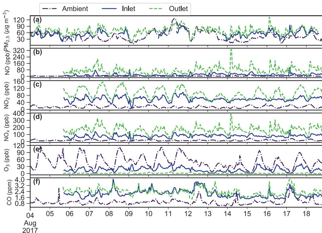
**Fig. 2.**  $PM_{2.5}$ ,  $NO$ - $NO_2$ - $NO_x$ ,  $O_3$ , and  $CO$  concentrations in the ambient air (represented by dash-dot lines) and at the inlet (represented by solid lines) and outlet (represented by dashed lines) of the WJL tunnel.
