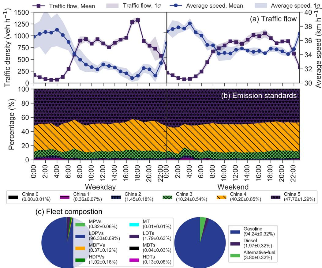
**Fig. 1.** Traffic characteristics (a: traffic flow including density and speed, b: emission standards, c: fleet composition) in the WJL tunnel during the measurement campaign.
