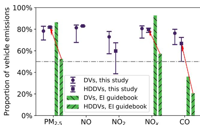
Fig. 6. Proportion of DV (diesel vehicle) and HDDV (heavy-duty diesel vehicle) emissions in the total on-road vehicle emissions from this study (represented by error bars with 95% confidence intervals) and 'EI guidebook' (represented by bars).
