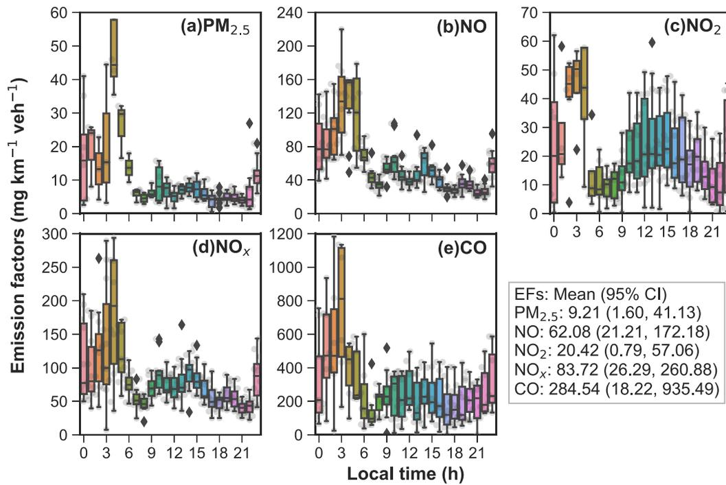
Fig. 3. Diurnal variations of average emission factors for PM<sub>2.5</sub>, NO-NO<sub>2</sub>-NO<sub>x</sub>, and CO from the fleet in the WJL tunnel.
